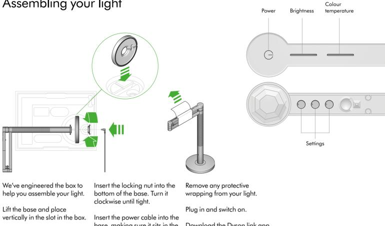
Insert the main body into the hole in the top of the base, making sure it's level.
