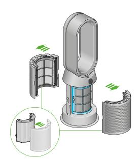
The air purifier and heater with the filter covers open showing a HEPA plus carbon filter located in the filter covers and a catalytic filter. Arrows demonstrate that the catalytic filter is fitted directly to the base of the machine and the filter covers will need to be assembled onto the base of the machine.
