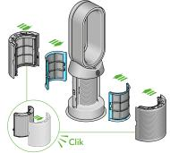
The air purifier and heater with the filter covers open showing a HEPA plus carbon filter located in the filter covers. Arrows demonstrate that the filter covers will need to be assembled onto the base of the machine.
