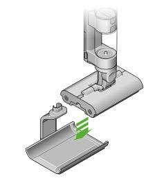
Using the menu button, scroll to Self clean using the blue button and select start.
